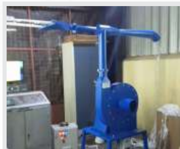
Trim Suction Unit
