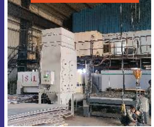
LASER SMOKE DUST COLLECTOR
